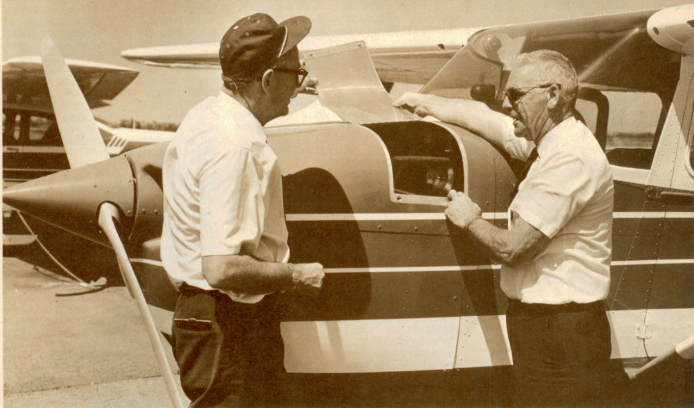
Keith Tobin (right), manager of Cessna's Fly-Away Division, points out left side access panel of new Skyhawk. Battery can be removed through here without taking off the cowling. Oil dipstick and fuel strainer are on the right side of Lycoming 150 h.p. engine introduced in this year's 172/Skyhawk series.
